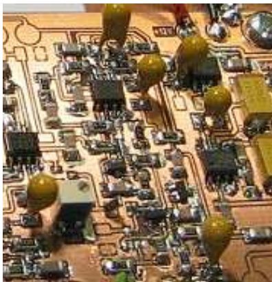
Fig. 11 – Using lead-type tantalum capacitors
